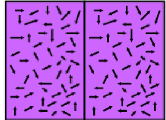
*Collisions transfer KE from hot to cold until equalized*
